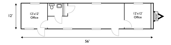
Note: This drawings represent design concept and general dimensions only. It is not intended to be used as a final construction drawing.
